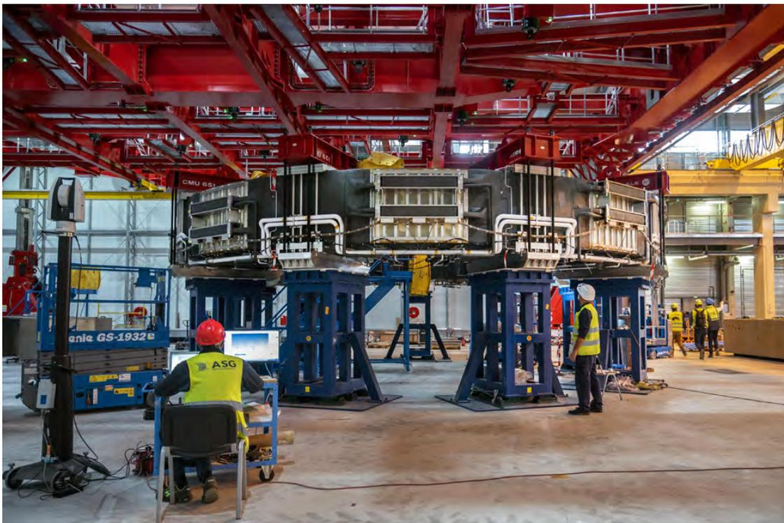
In April, the fifth poloidal field coil will be completed. It's the first to be entirely manufactured on-site.
